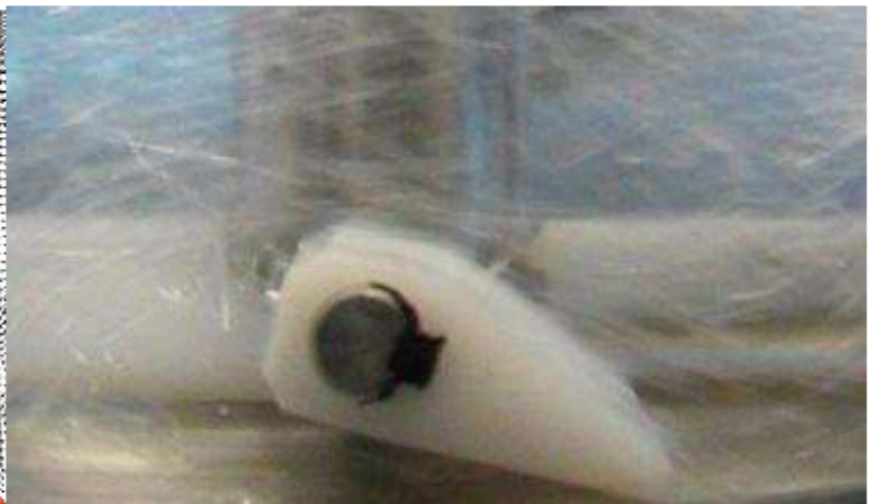
Figure 6. Particle trajectories from particle-flow simulations for the streamlined scraper geometry compared to measured particle-flow visualization. The top two figures correspond to 20 seconds after start up, and the bottom two to 230
